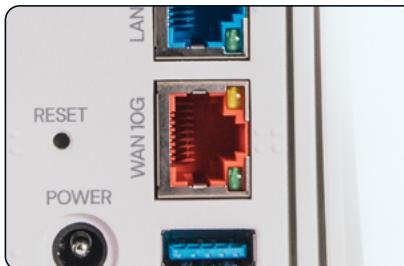
Plug one end into the WAN port on the Hub and the other end into the fibre connection box (ONT).
