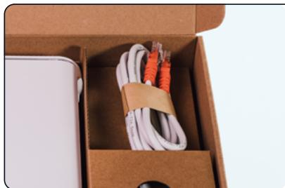
The Hub should always be connected to our fibre connection box (ONT) with the Ethernet cable that came with it.
